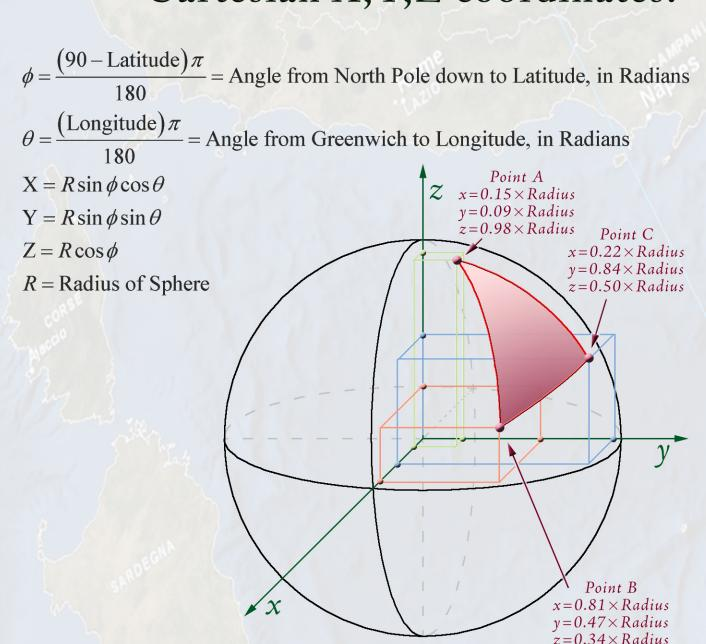
Step 3: Calculate the 3D centroid of the 3 triangle vertices, and then shift that point out to the surface of the planet.
