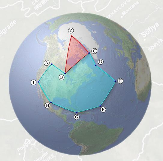
Step 3: Note direction of the triangle vertices. The vertices for  $\triangle BCZ$ above are entered in a counterclockwise direction, so the area for  $\triangle BCZ$  is set to negative.
