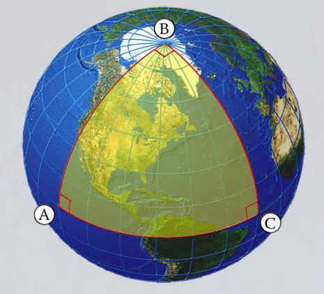
Triangle area can easily be calculated using either triangle side lengths or internal angles. Internal angles of a spherical triangle always exceed 180°, and this "spherical excess" is directly related to the triangle area.
