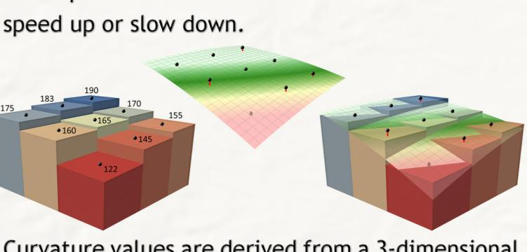
Curvature values are derived from a 3-dimensional polynomial curve fitted to the 9 elevation points. This extension uses a 6-parameter polynomial to model the surface (see manual for details).
